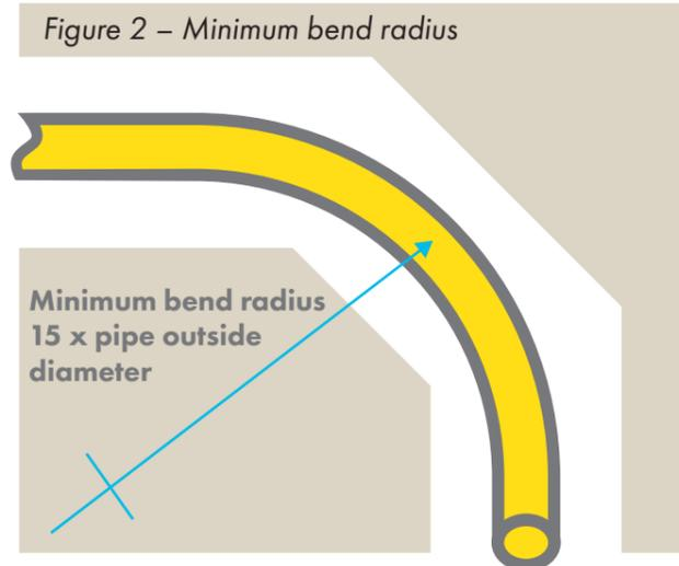
If it is necessary to lay pipe/ducting around bends, Tables 1 and 2 should be followed to ensure that the minimum bend radius is not exceeded.
